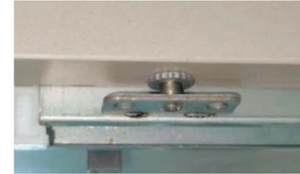
Adjusting nut on underside of drawers
